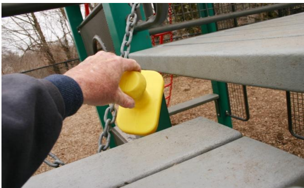
Metal Composite Structure- Chain Funnel Bridge- 4 Head Entrapments- Class A Hazard
