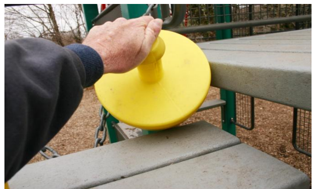
Metal Composite Structure- Chain Funnel Bridge- 4 Head Entrapments- Class A Hazard
