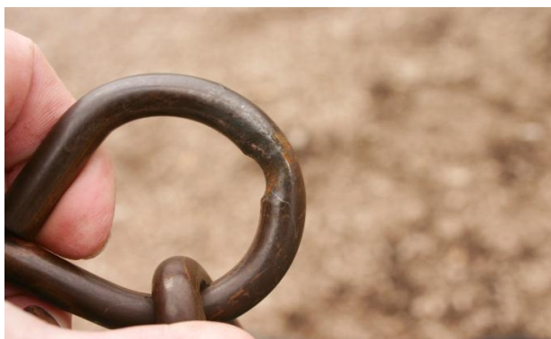
2 Bay Tot Seat Swing Set- "S" Hooks and Chains Worn- Class A HAZARD
