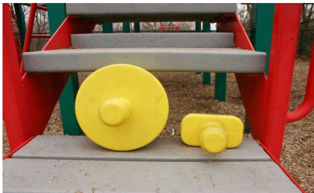
Metal Composite Structure- Stairs- Head Entrapment- Class B Hazard
