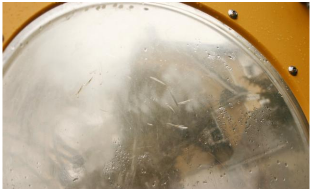
Large Composite Structure- Bubble Panel- Cuts in Plastic Bubble - MAINTENANCE
