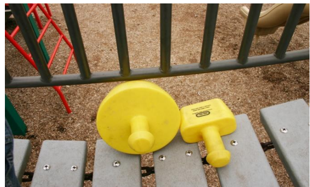
Metal Composite Structure- Suspension Bridge- 2 Head Entrapments- Class A Hazard
