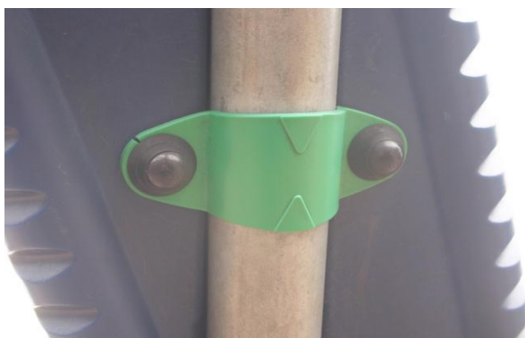
Antares Galaxy Climber- Cracks in plastic brackets- MAINTENANCE
