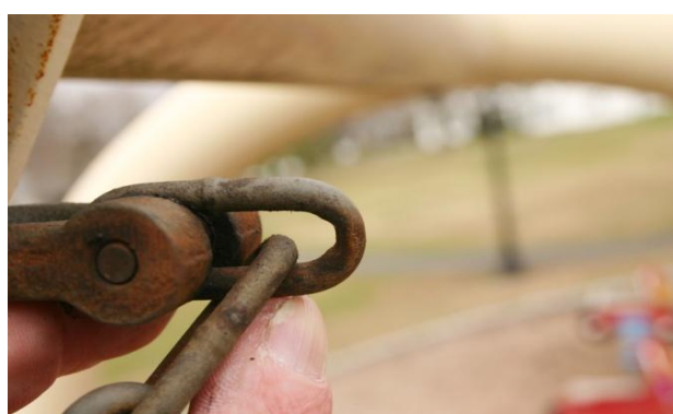
2 Bay Tot Seat Swing Set- "S" Hooks and Chains Worn- Class A HAZARD
