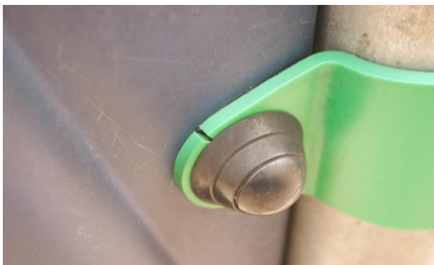
Spica Whirl Rider- Fabric Exposed- Class B HAZARD
